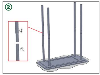
Connect the Pipe #1 and #2, inserting them into the slots in base
